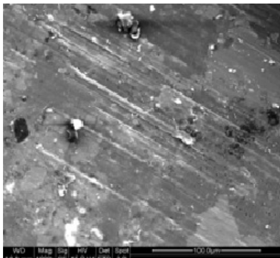
Fig 3 SEM image of fretting scar
