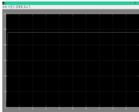
Figure 6(f).Output voltage of PV module after MPPT
